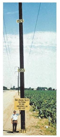
Figure 1. Approximate location of maximum measured subsidence (9 m) in the San Joaquin Valley, California (1925–77) attributed to aquifer-system compaction caused by groundwater abstraction. Signs on pole (1925, 1955) are positioned at approximate former elevations of land surface. Pictured is Dr. J.F. Poland; photograph by R.L. Ireland, USGS, *ca.* 1977.
